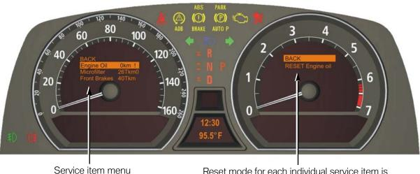
Reset mode for each individual service item is entered by pressing item in menu for greater than 2 seconds The residual wear or the remaining time are specified (possibly with a minus sign).
